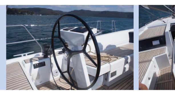
**LEFT TO RIGHT**: Port side you can see the twin winches, the repeater navigation instruments and the lift up seat covering the rope tail bag.
