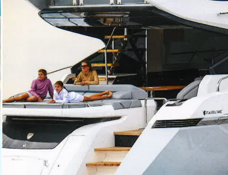
Aft moulding lifts to reveal tender garage. Opening sections are for shower, bench and cover storage
