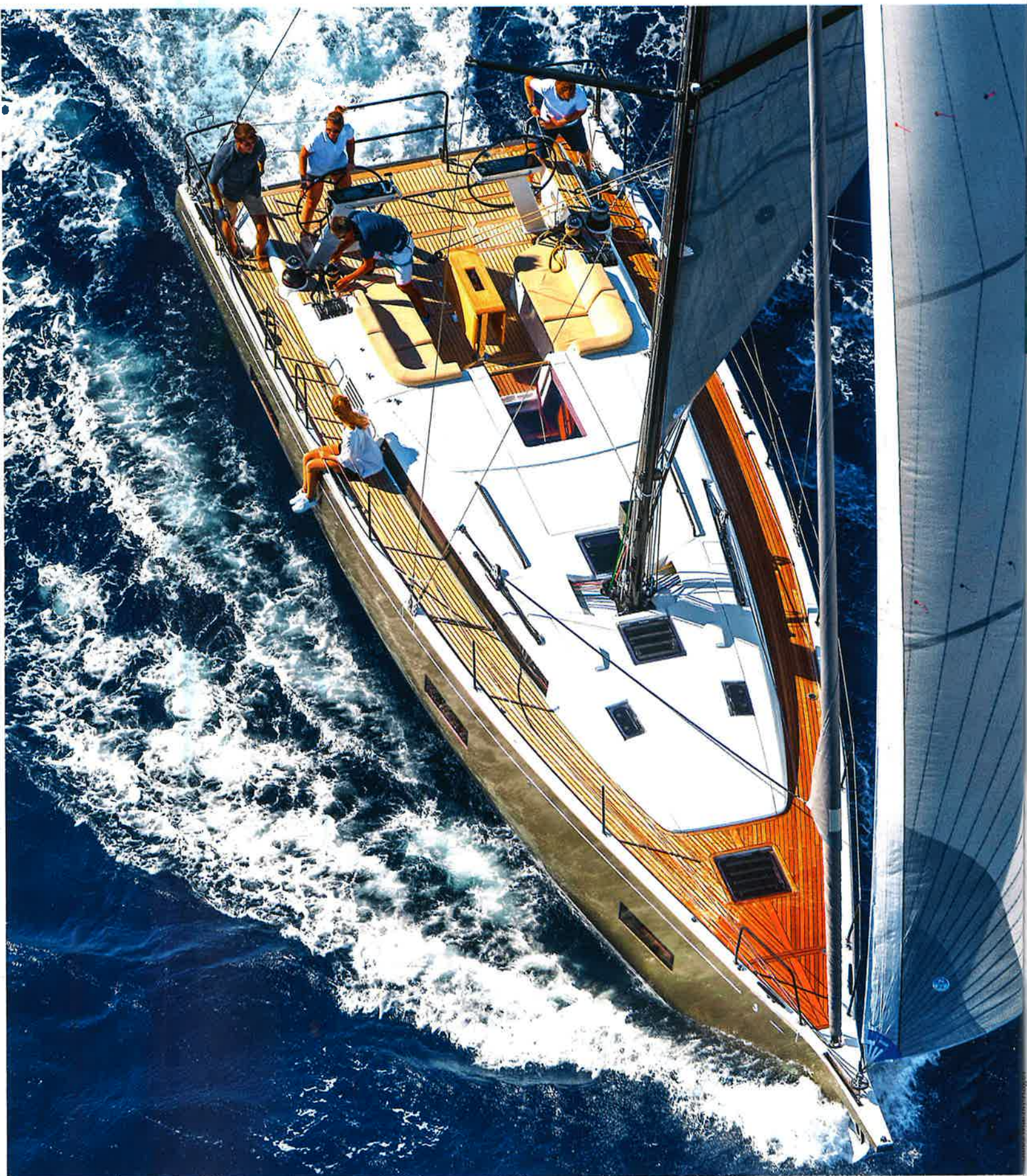
Powerful shape for offwind sailing: bowsprit can fly both an asymmetric spinnaker and a Code 0 (shown)
