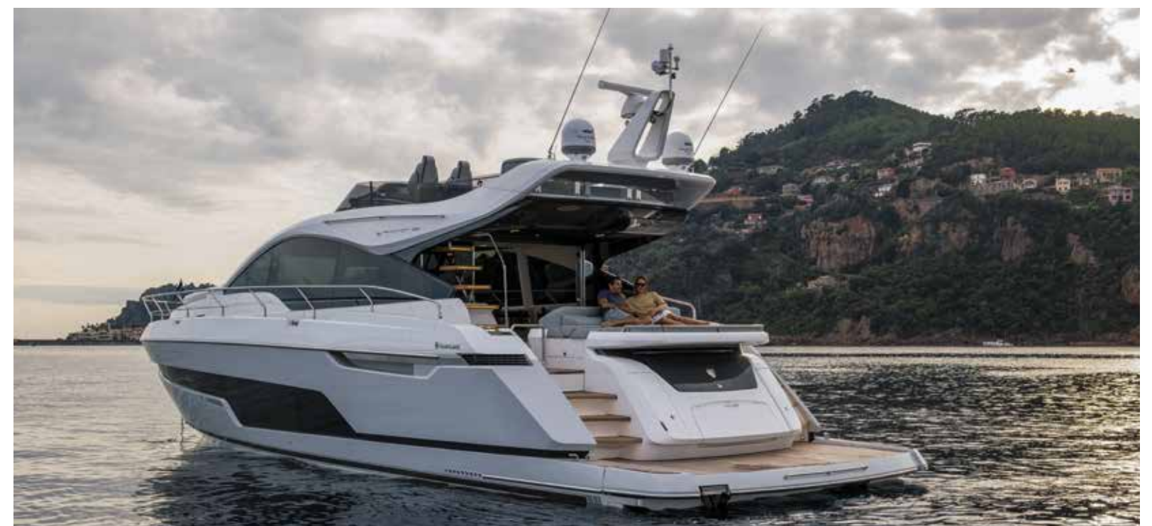
The aft platform has a 400kg-lifting capacity, the garage can house a Williams 345 SportJet, while the garage door features a fold-out sofa
