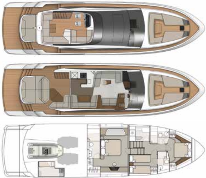
Note: Lower deck shows three-cabin layout with utility room; port room can be a bunk cabin, day head or en-suite bathroom for extended VIP cabin
