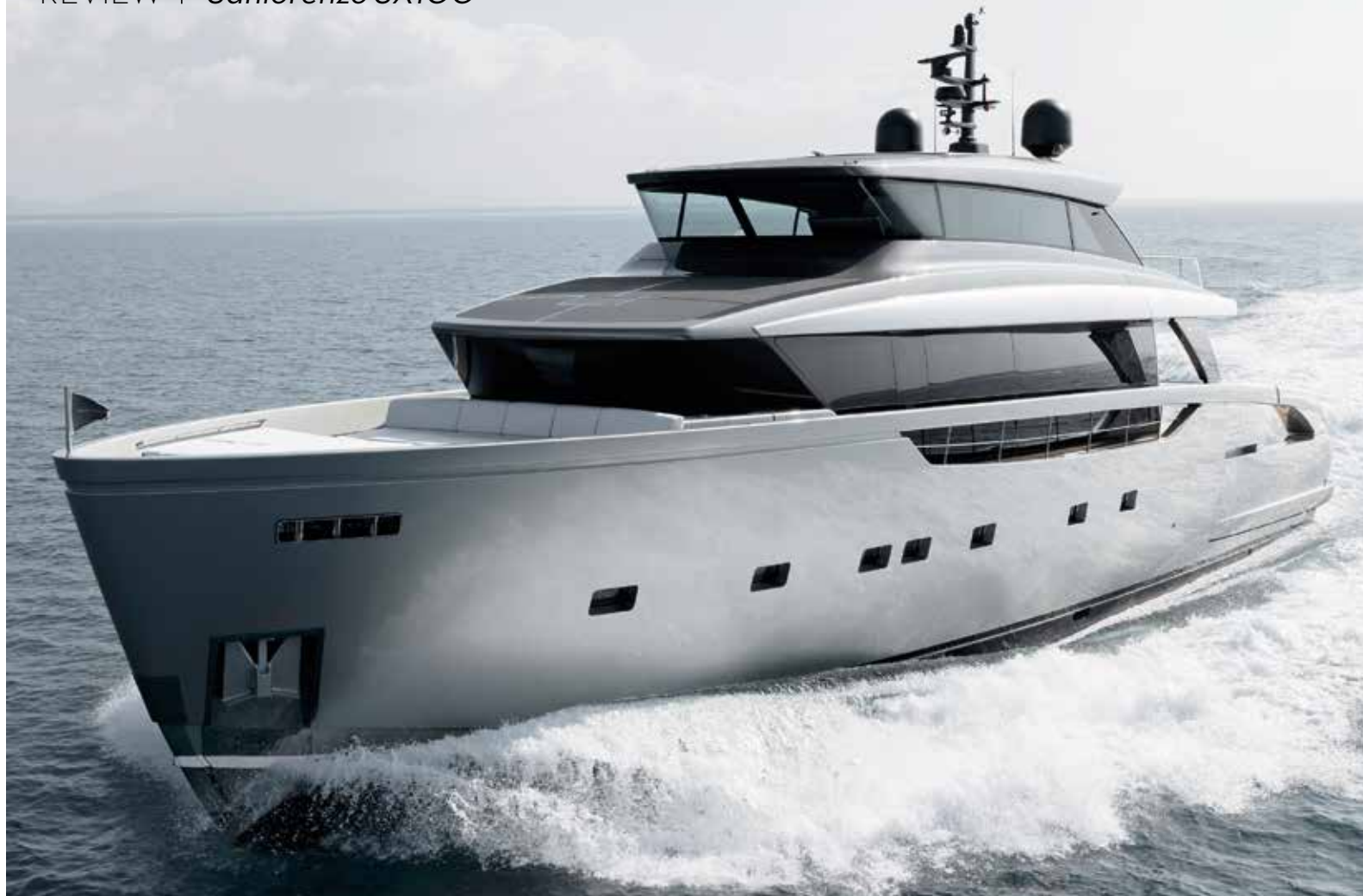
Distinguished by reverse-angled windscreens, the SX100 has a planing hull and a top speed of 23 knots with four 800hp Volvo Penta IPS pod drives
