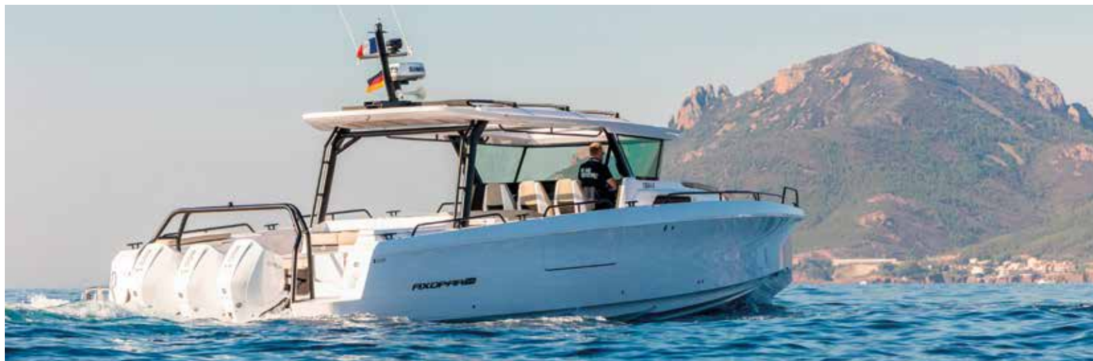
The Axopar 45 is powered by triple 300hp Mercury Verado V8 outboard engines, delivering highly efficient cruising between 22 and 34 knots
