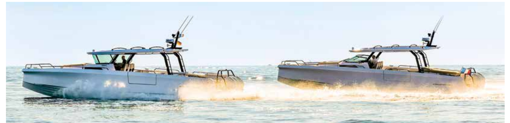
The semi-enclosed Cross Top version has a reverse-angle windscreen, while the Sun Top, shown with the aft cabin option, offers a breezier ride
