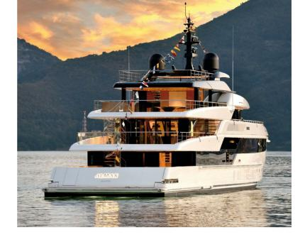
The 49.99-metre yacht is the world's first superyacht to accommodate the modular Reformer Fuel Cell system, developed in collaboration with Siemens Energy, capable of transforming methanol into hydrogen and then into a maximum of 100kW of electrical energy to power all the yacht's hotel systems without the need to store space-consuming hydrogen on board, and with propulsion engines and diesel generators turned off.
