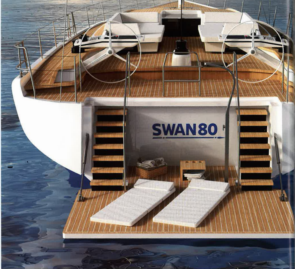
Above: The Swan 80's full beam lazarette can accommodate a rigid inflatable tender
