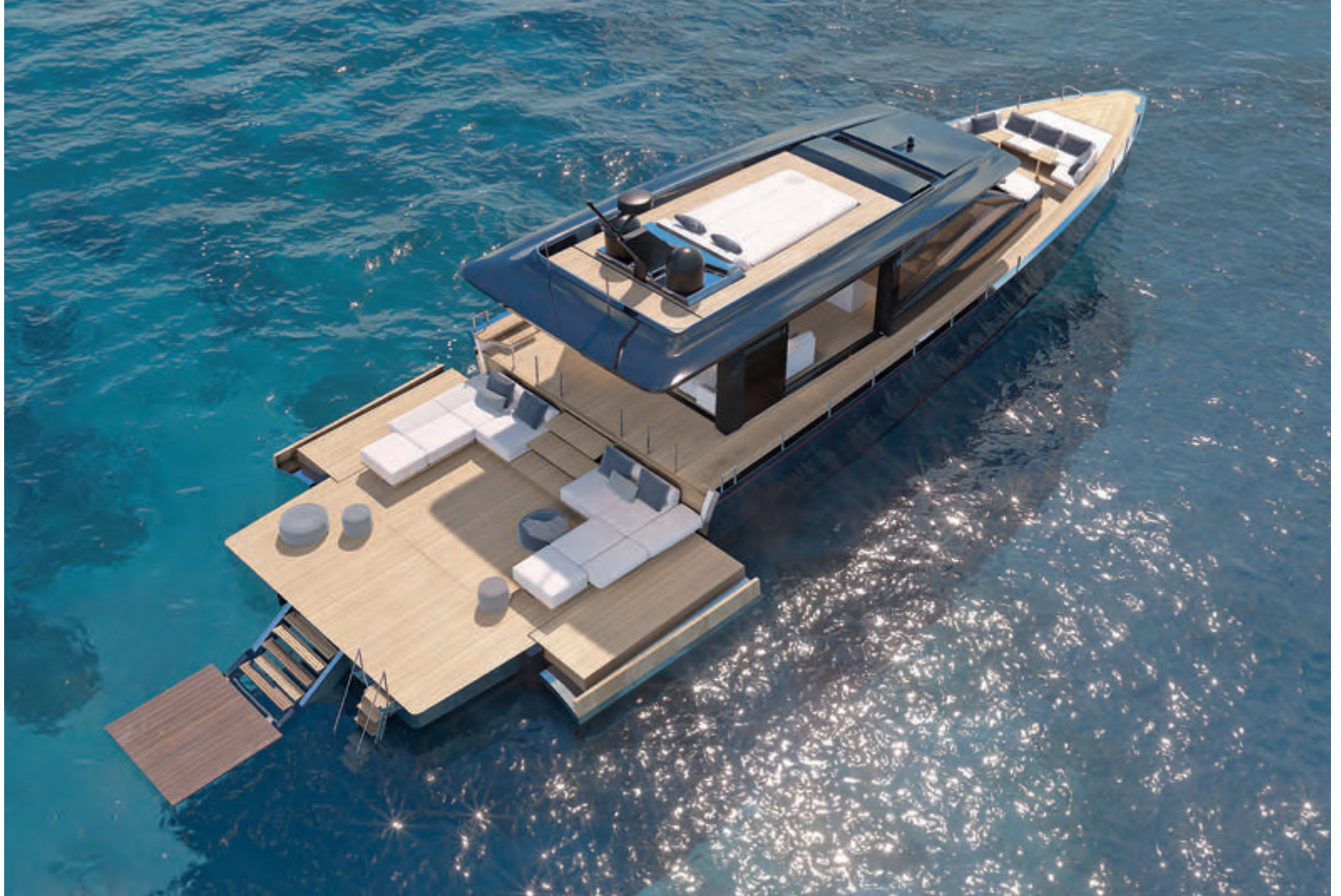
The split-level main deck culminates in an extending swim platform with folding bulwarks to create a 50sqm area (also shown at bottom right of page)
